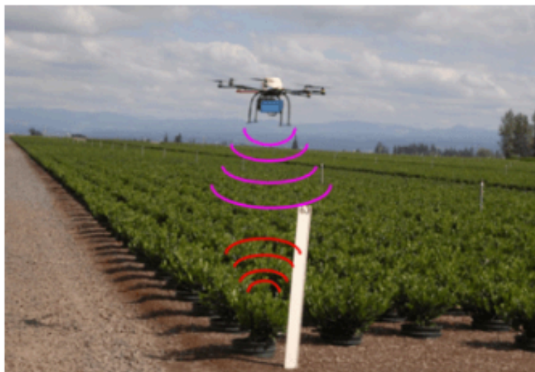
Fig. 3. Merging RFID tags with a sUAS for plant inventory.
