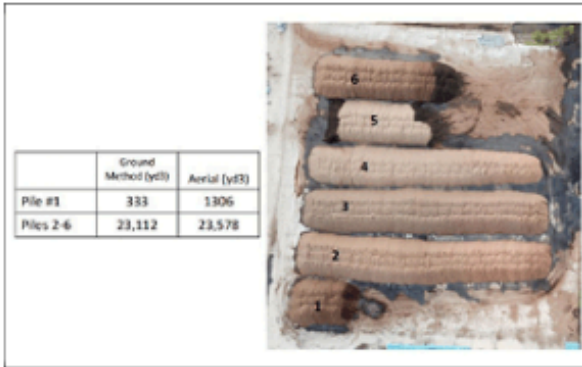
Fig. 1. Example of preliminary work we conducted using an inexpensive drone and processing the images using DroneDeploy service to estimate the volume of bark piles.
