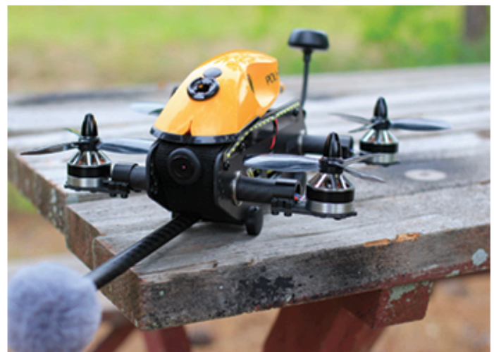
North Carolina company OpenRobotix Labs' Poli-X1 is equipped with a proboscis in its front that it uses to transfer pollen.
